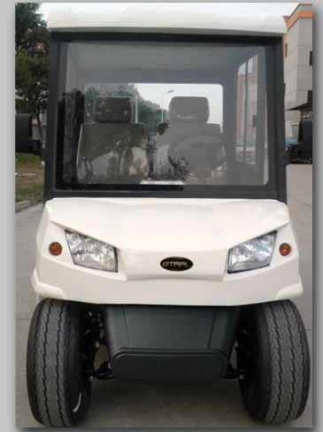
Plastic-covered, steel-reinforced bumper
