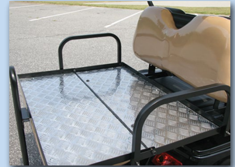
Flip seat with aluminum plate
