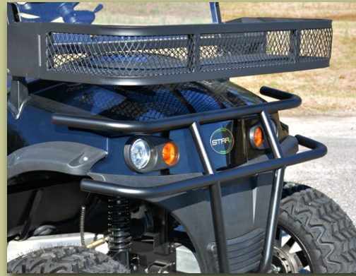
Fully loaded with black powder-coated stainless steel brush guard and clay basket
